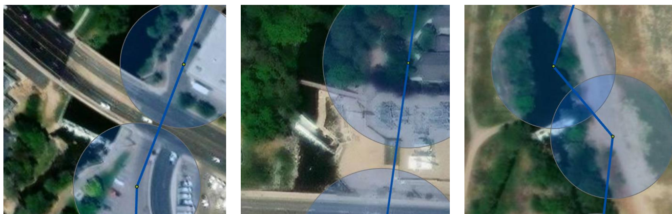
Figure 12. Examples of misplaced Hydrofabric flowlines (Blue lines).
