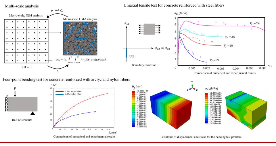
Multi-Scale Modeling of Fiber-Reinforced-Concrete Structures using Granular Micromechanics Approach
