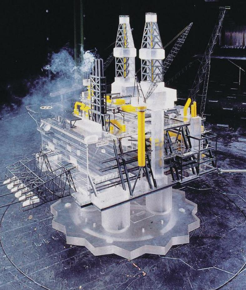
30 mph. According to the Canadian Society for Civil Engineering, “The adjustable roof height allows accurate simulation of pressure gradients, and the long test section allows turbulent boundary layer flow to naturally develop over roughness elements on the wind tunnel floor.”
